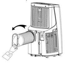
2. Attach the connector on the opposite end of the pipe to the exhaust outlet on the rear of the appliance by putting it into position and twisting to lock in place
