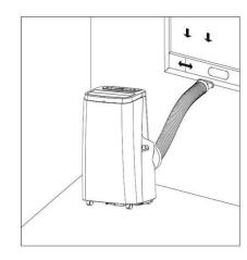
2. Fix the fishtail on the hose into the opening in the slide bar.
